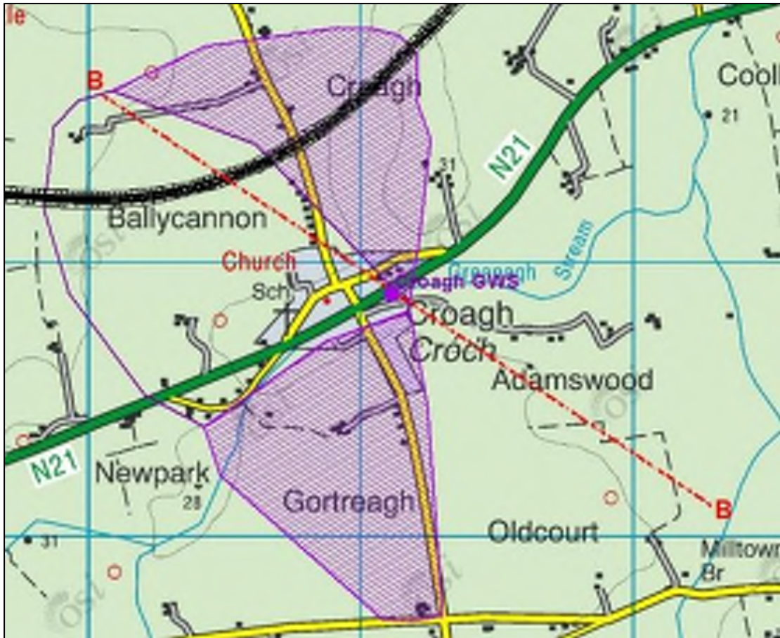
Plate 9.8 Zone of Contribution (in Purple) with additional potential contribution areas (hatched Purple) at Croagh area (refer to Plate 9.9 for section B-B and CSM)
