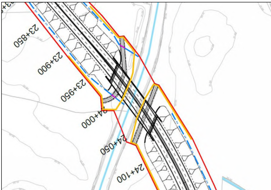
Plate 6.16 River Deel silt fencing provision at Ch. 24+000
