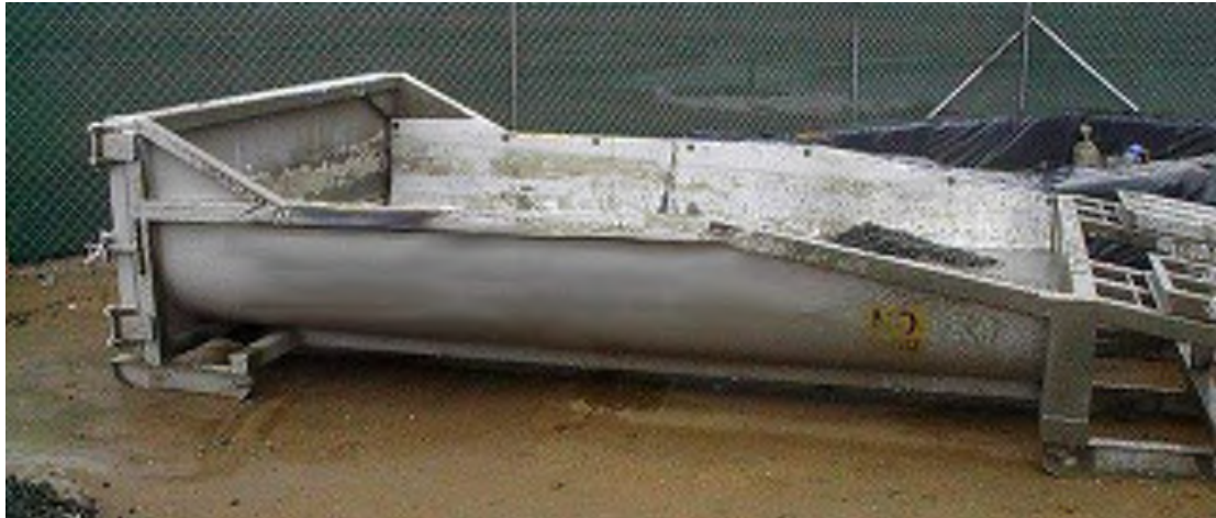
Plate 6.6 Typical washout facility
